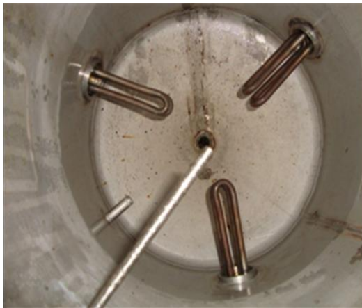
Fig.4 Arrangement of electric heating element
